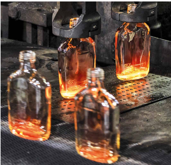
Production of Hennessy V.S. flasks in the Verallia electric furnace in Cognac.
